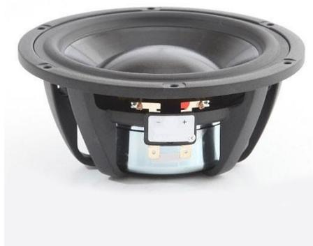
The Midrange/Woofer's former (bobbin) is made of titanium for smoother more extended dynamics, power handling, and frequency response. Titanium's added stiffness also allows for a larger voice coil. The voice coil is 3.1 inches in diameter. Titanium is an expensive and difficult material to work with, but well worth it for the increase in quality and performance.
